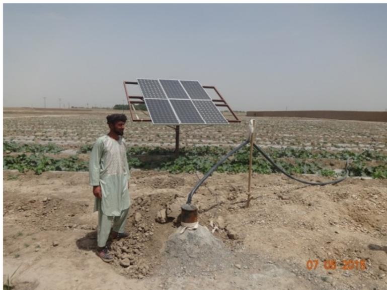
Solar panel used for powering pump irrigation, Afghanistan. Source: MCN/UNODC
